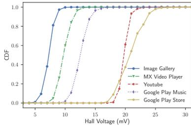
Figure 2: CDF of MF values for 5 apps to validate energy consumption
