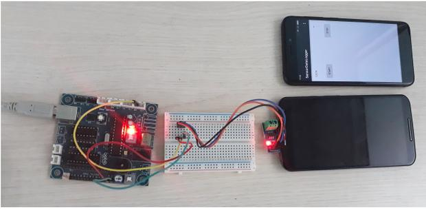
**Figure 1: Experimental in-laboratory setup: The Hall sensor connected to an Arduino board collects Hall effect values, while a Moto X2 phone collects magnetometer values from the target smartphone.**
